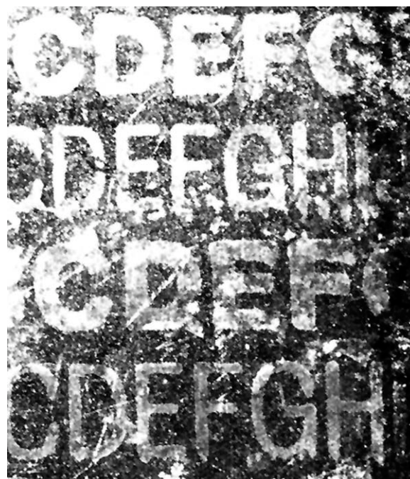
Plate 2 Imaged Cu plate using poly(GMA-co-AA) resist with 25 mol % AA after exposure to UV light and before development.
